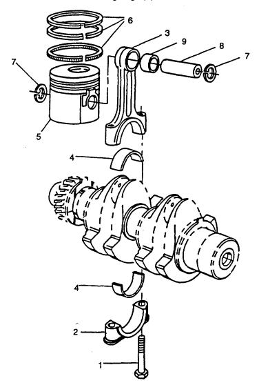
FIGURE 3-36. Piston and Connecting Rod Assemblies
