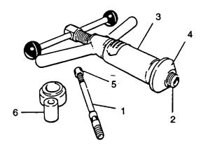
FIGURE 3-29. Valve Guide Tool and Depth Stop
