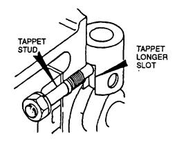
FIGURE 3-8. Fuel Pump Tappet and Stud
