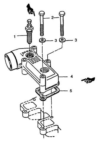
FIGURE 3-2. Intake Manifold
