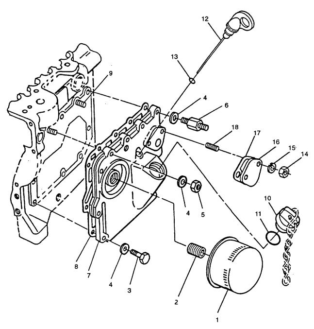
FIGURE 3-15. Oil Filter and Crankcase Door
