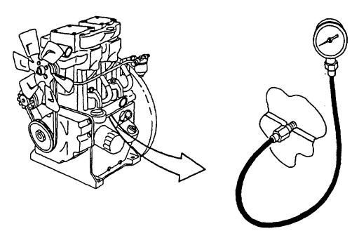
FIGURE 3-18. Oil Pressure Test Setup
