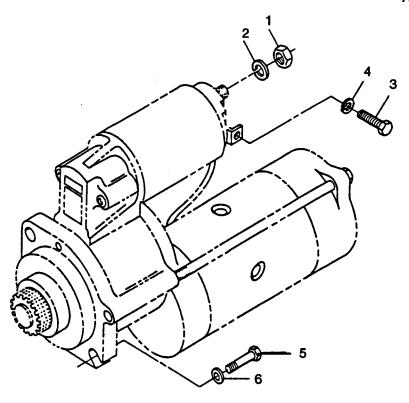
FIGURE 3-21. Starter Connection and Mounting Hardware
