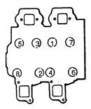
FIGURE 3-31. Cylinder Head Bolt Tightening Sequence
