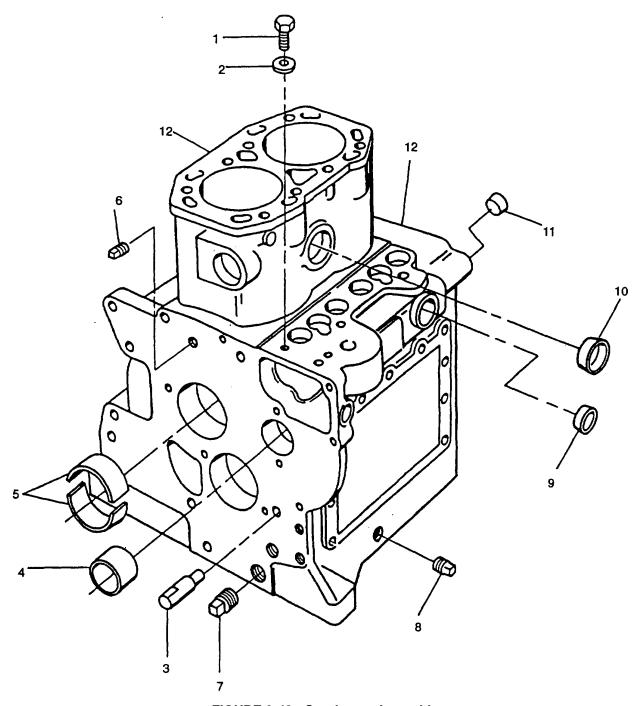
FIGURE 3-43. Crankcase Assembly
