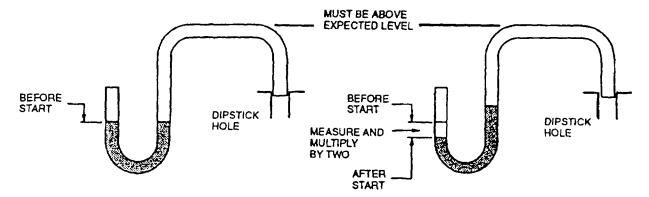
FIGURE 3-1. Locally Manufactured Water Manometer
