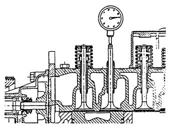
FIGURE 3-10. Checking Piston Drop
