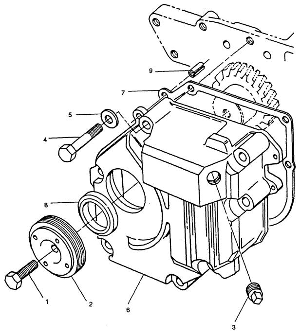
FIGURE 3-32. Gear End Cover
