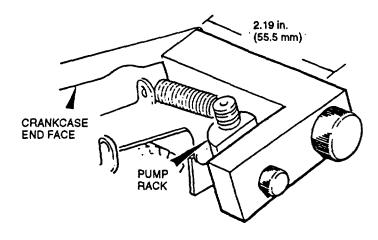
FIGURE 3-9. Setting Pump Rack
