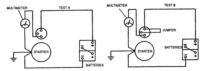
FIGURE 3-23. Starter Solenoid Test Circuit
