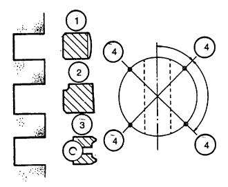
FIGURE 3-37. Piston Ring and Gap Location
