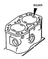
FIGURE 3-30. Checking Cylinder Head Clearance
