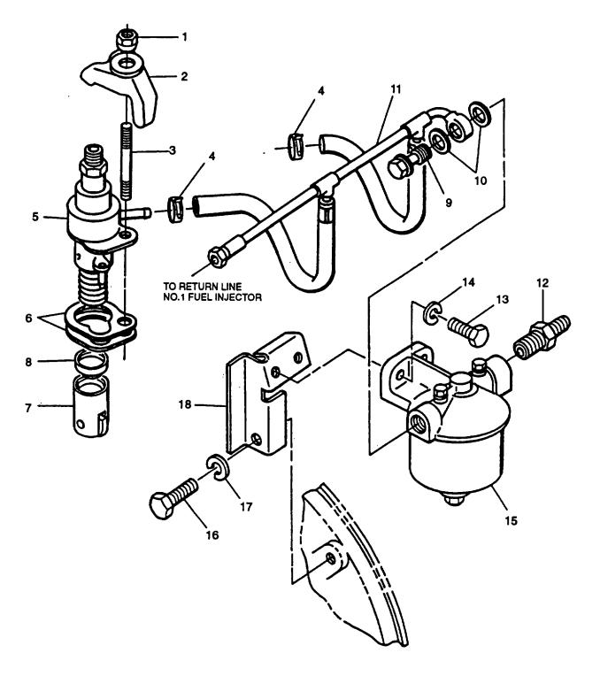
FIGURE 3-7. Fuel Injection Pump, Fuel Filter, and Supply Lines
