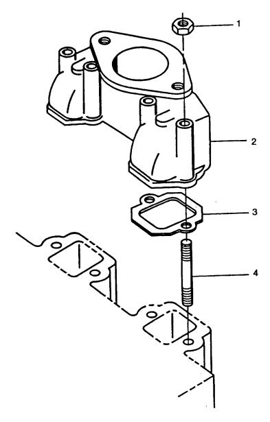
FIGURE 3-3. Exhaust Manifold
