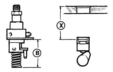
FIGURE 3-11. FUEL INJECTOR Pump Dimensions
