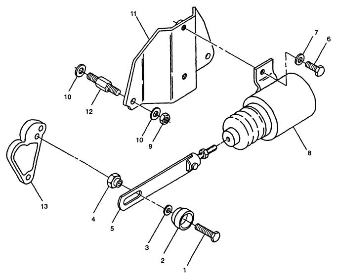
FIGURE 3-14. Fuel Solenoid Installation
