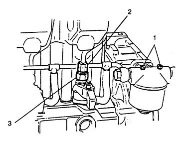
FIGURE 3-5. Priming Fuel System
