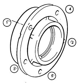
FIGURE 3-42. Bearing Housing Capscrew Tightening Sequence CAUTION
