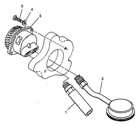
FIGURE 3-17. Strainer and Oil Pump
