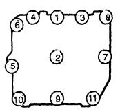
FIGURE 3-16. Crankcase Door Fastener Tightening Sequence
