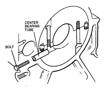
FIGURE 3-39. Center Bearing Tube
