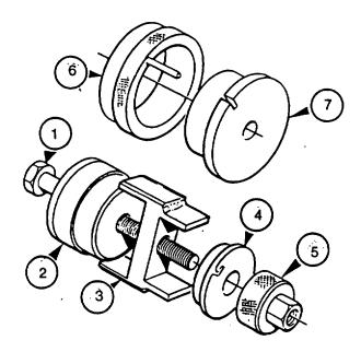
FIGURE 3-41. Main Bearing Tool
