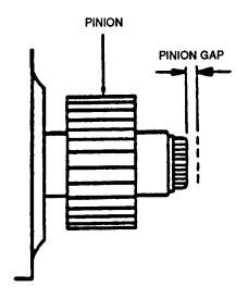
FIGURE 3-26. Checking Pinion Gap
