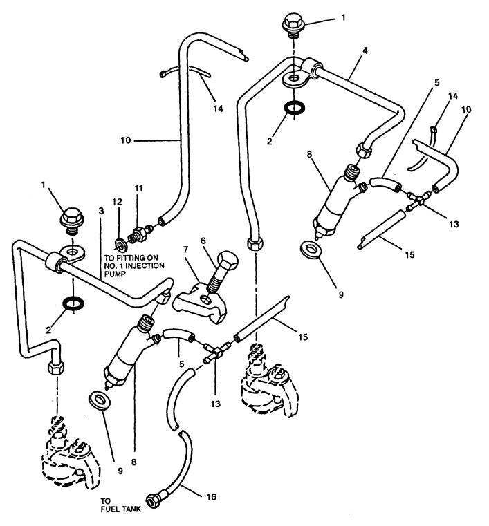
FIGURE 3-13. Fuel Infectors, Fuel Injector Pipes, and Fuel Return Line 3-32
