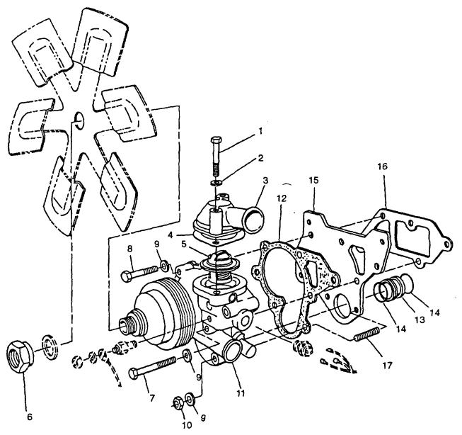
FIGURE 3-4. Cooling System
