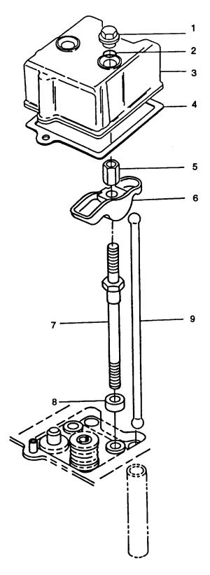
FIGURE 3-27. Cylinder Cover and Rocker Lever
