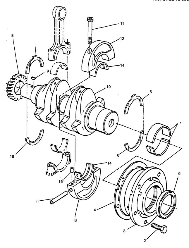
FIGURE 3-40. Crankshaft Assembly
