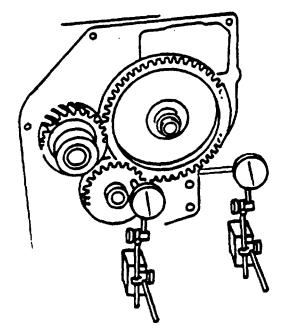
FIGURE 3-35. Measuring Gear Backlash and End Play
