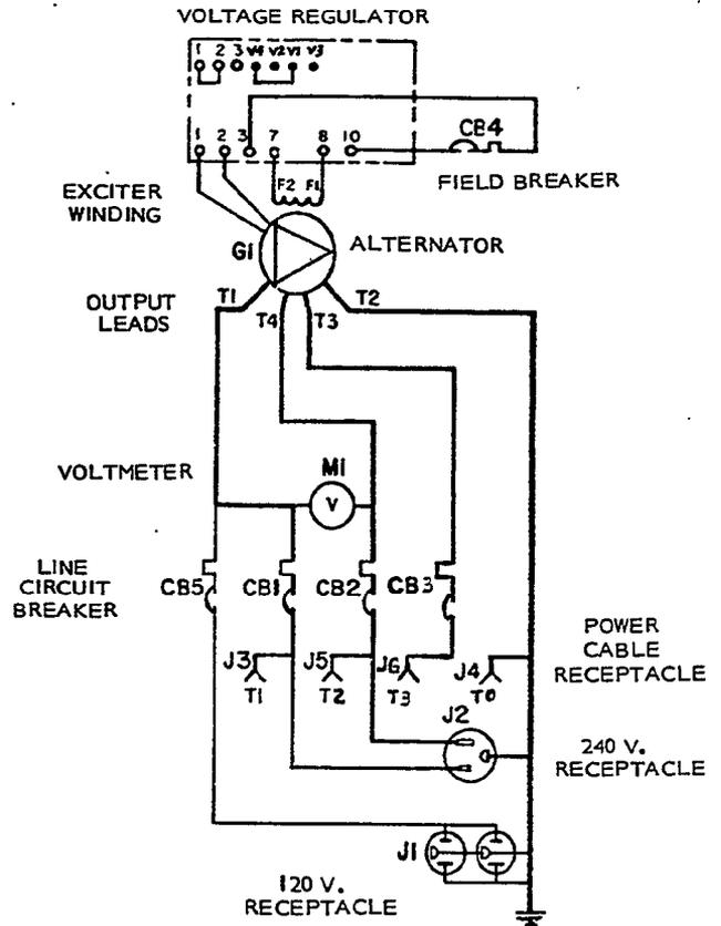
FIGURE 42. THREE PHASE 240 VOLT DELTA CONNECTIONS
