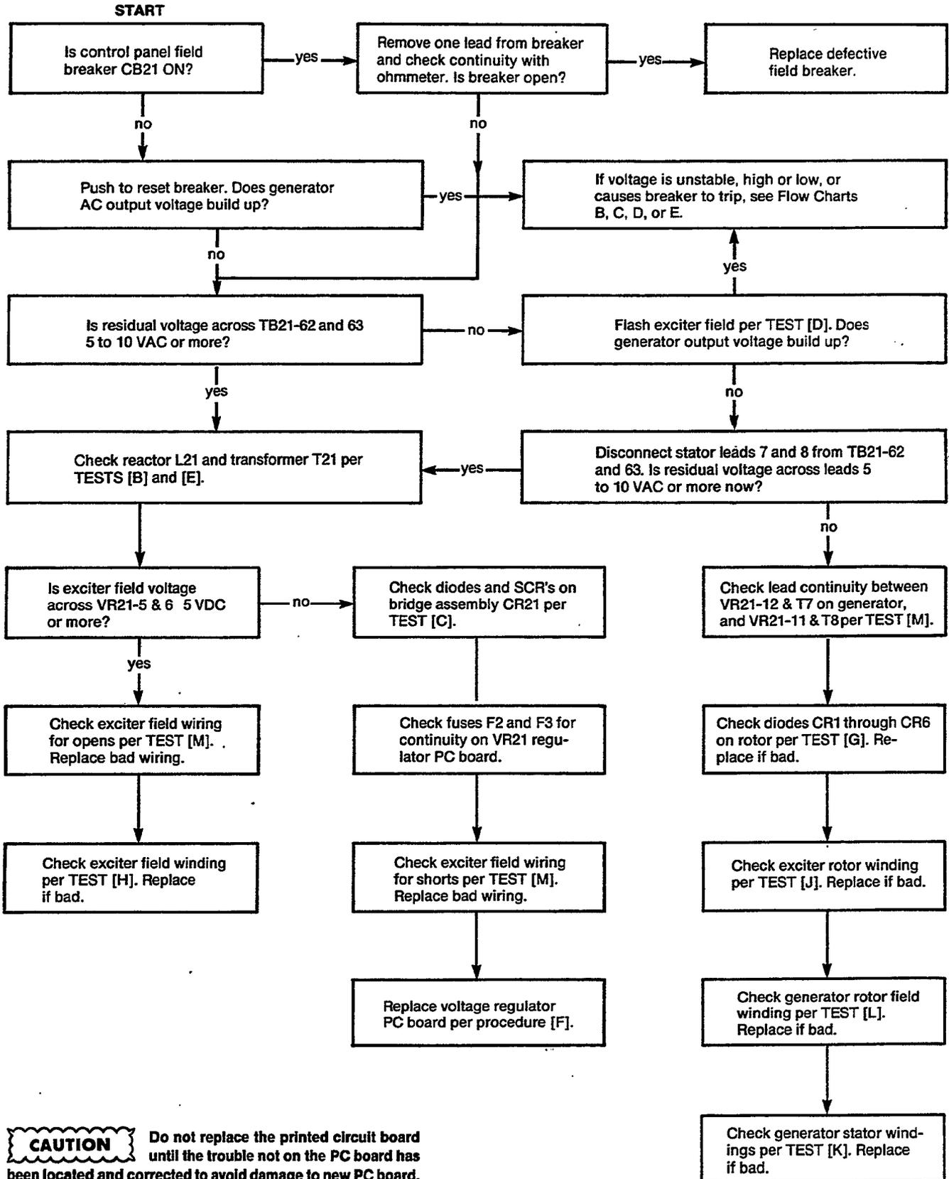
**CAUTION** Do not replace the printed circuit board until the trouble not on the PC board has been located and corrected to avoid damage to new PC board.
