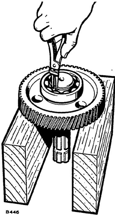
**FIGURE 53. INSTALLING SNAP RING BEHIND DRIVE GEAR BEARING**
