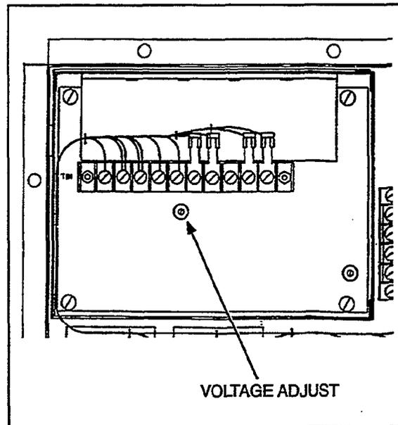
FIGURE 10. VOLTAGE REGULATOR BOARD
