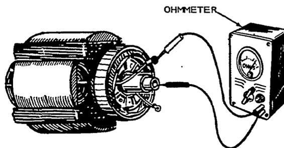
CONTACT ONE PROD TO EACH OF THE FIELD LEADS AND OTHER PROD TO ROTOR SHAFT. IF ROTOR IS GOOD, THERE WILL BE NO READING ON OHMMETER.
