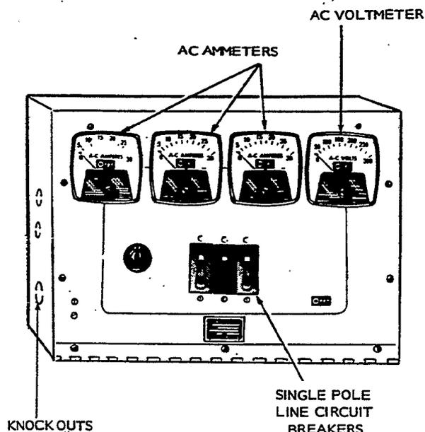
FIGURE 46. TYPICAL WALL MOUNTING "SB" SWITCHBOARD - 3 PHASE, 120/208 VOLTS
