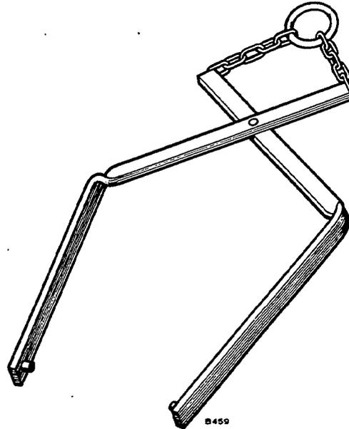
FIGURE 58. STATOR HANDLING TONGS
