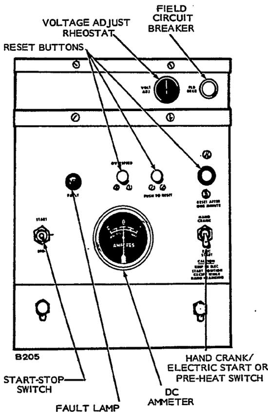
FIGURE 69. TYPICAL AIR-COOLED AND MARINE SET CONTROL PANEL
