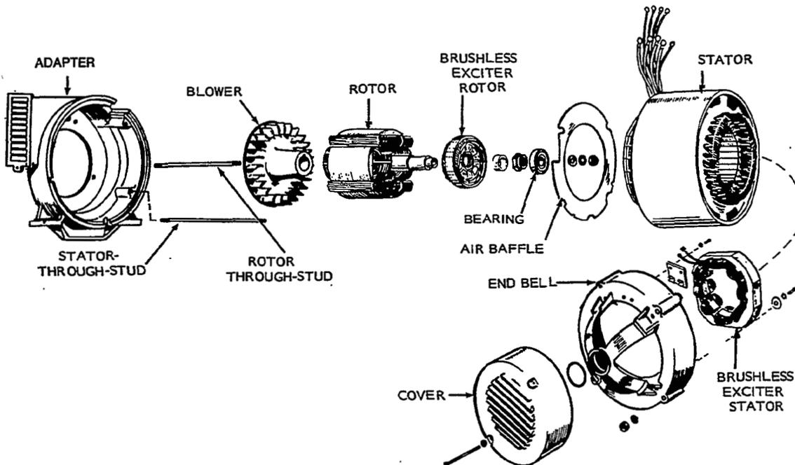
FIGURE 38. GENERATOR DISASSEMBLY
