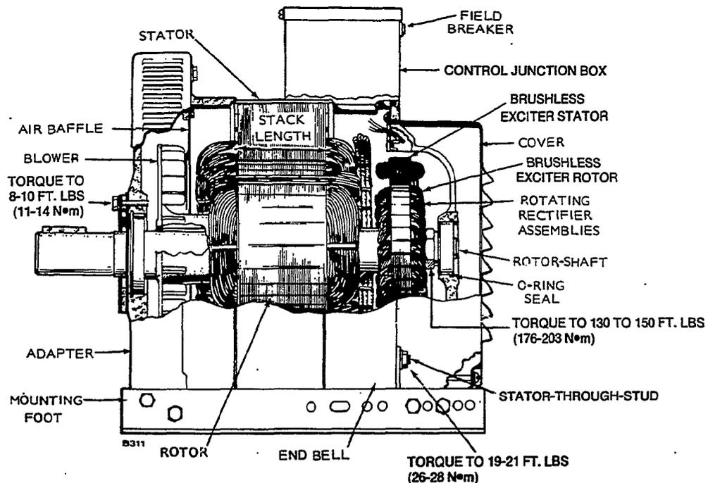
FIGURE 44. GENERATOR (CUTAWAY VIEW)
