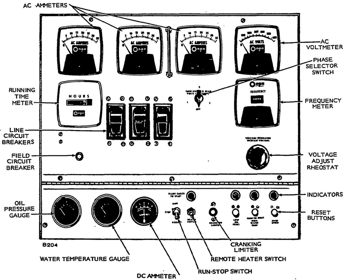
FIGURE 71. TYPICAL RADIATOR-COOLED SET CONTROL PANEL
