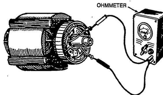
CONTACT ONE PROD TO ONE FIELD LEAD AND OTHER PROD TO OTHER FIELD LEAD. RESISTANCE VALUES ARE GIVEN IN TABLES 2 AND 4.
