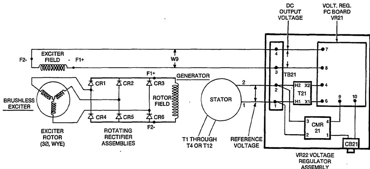
FIGURE 4. ELECTRICAL SCHEMATIC, STANDARD YD GENERATOR AND REGULATOR
