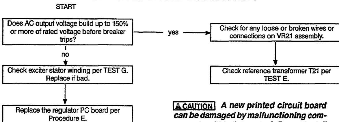
**CAUTION** A new printed circuit board can be damaged by malfunctioning components within the control. Do not install the new PC board until all other problems have been located and corrected.
