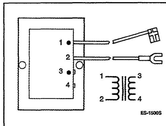
FIGURE 1. COMMUTATING REACTOR
