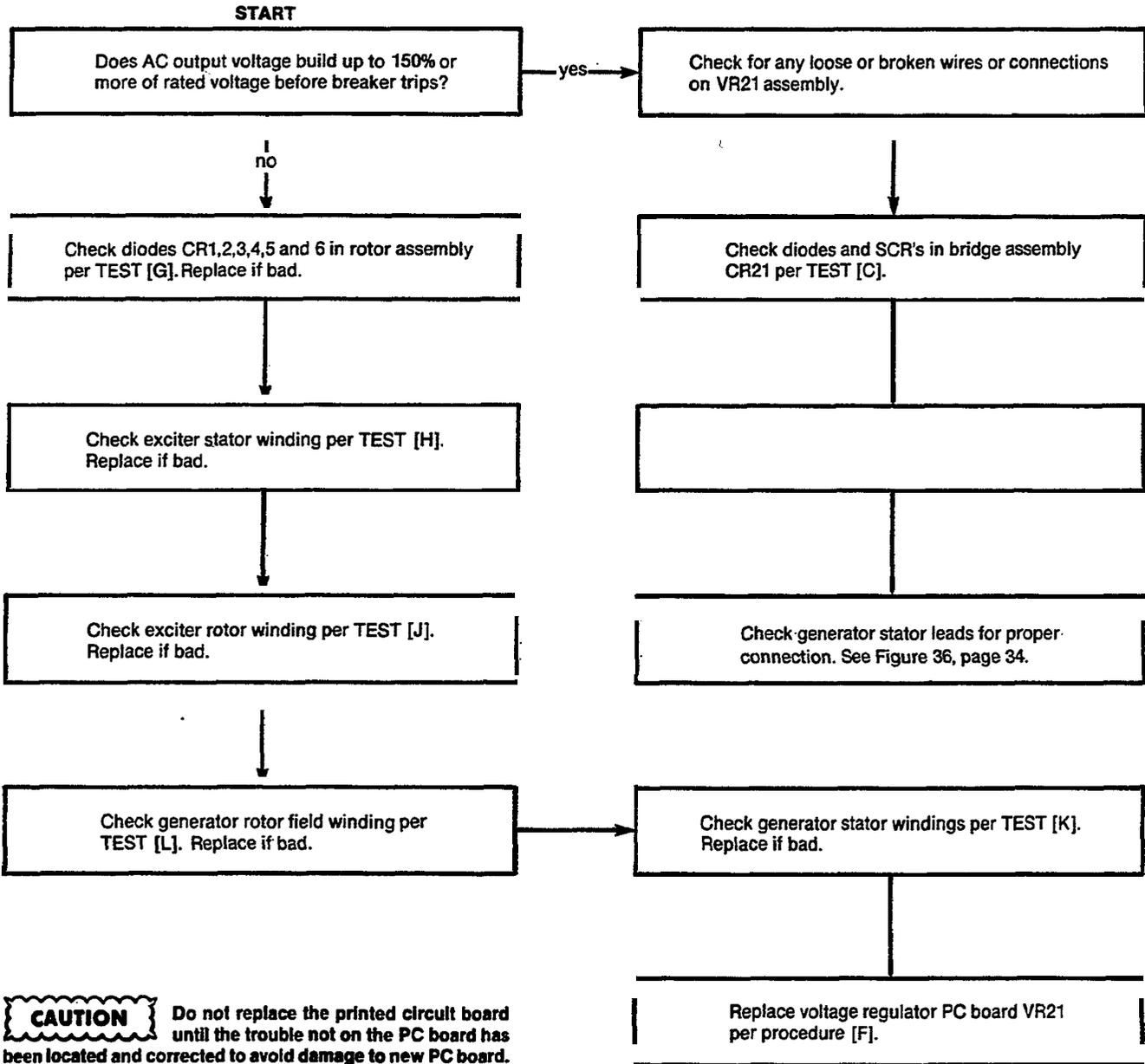
**CAUTION** Do not replace the printed circuit board until the trouble not on the PC board has been located and corrected to avoid damage to new PC board.
