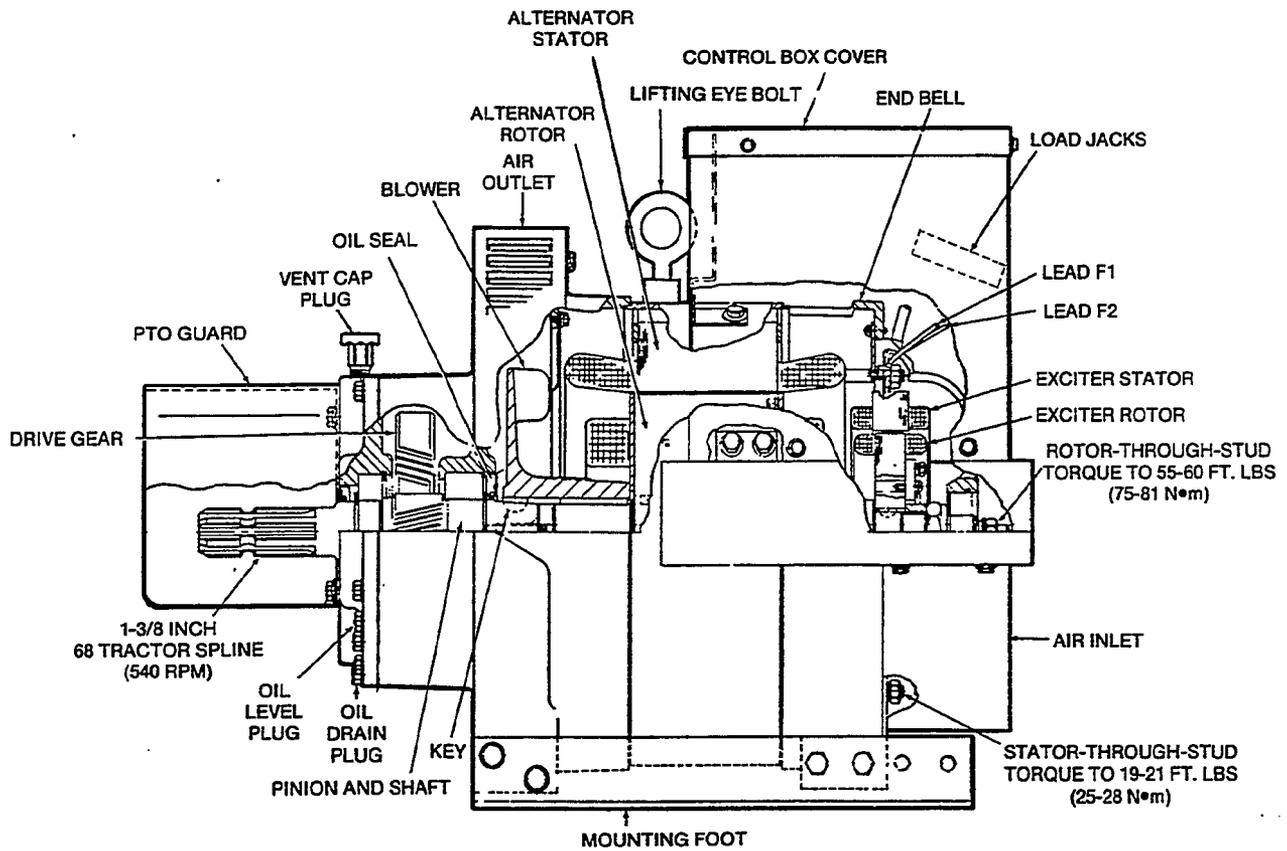
FIGURE 40. YD TRACTOR DRIVE ALTERNATOR
