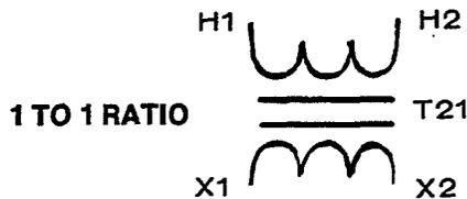
Resistance between H1-H2 should be 113 to 139 ohms, between X1-X2 133 to 163 ohms at 77° F (25° C). Resistance between coils and from any terminal to transformer frame should be infinity.
