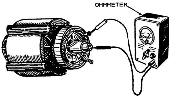
CONTACT ONE PROD TO EACH OF THE FIELD LEADS AND OTHER PROD TO ROTOR SHAFT. IF ROTOR IS GOOD, THERE WILL BE NO READING ON OHMMETER.
