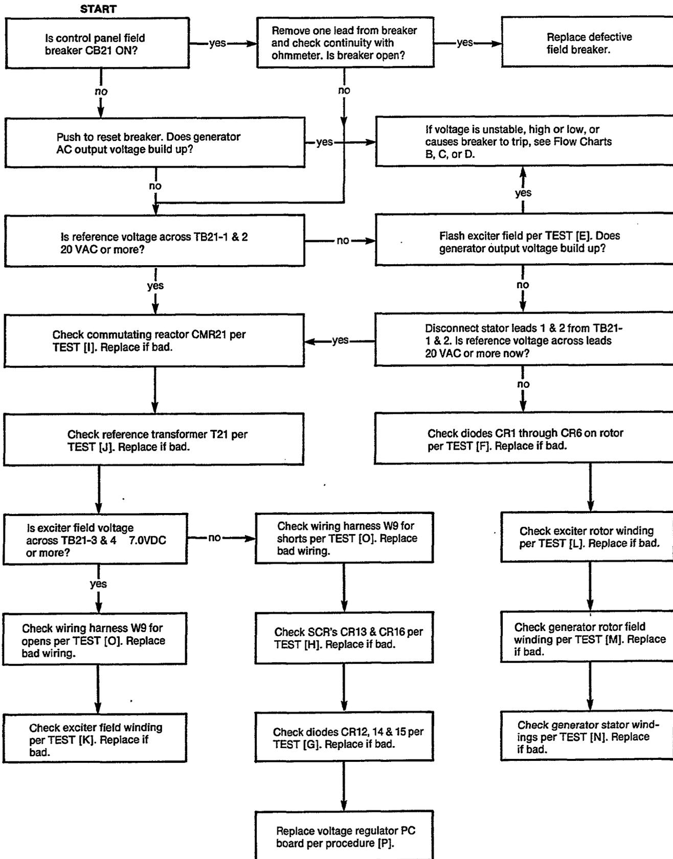
**CAUTION** Do not replace the printed circuit board until the trouble not on the PC board has been located and corrected to avoid damage to new PC board.
