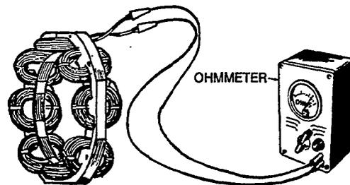
OHMMETER RESISTANCE BETWEEN F1 AND F2 SHOULD BE 10.98 TO 13.42 OHMS
