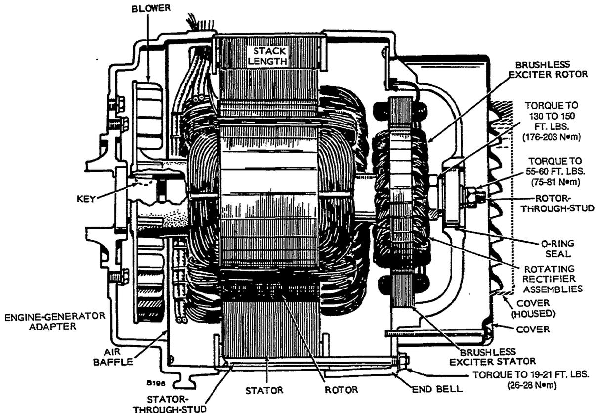
FIGURE 1. TYPICAL YD J-SERIES GENERATOR (SECTIONAL VIEW)
