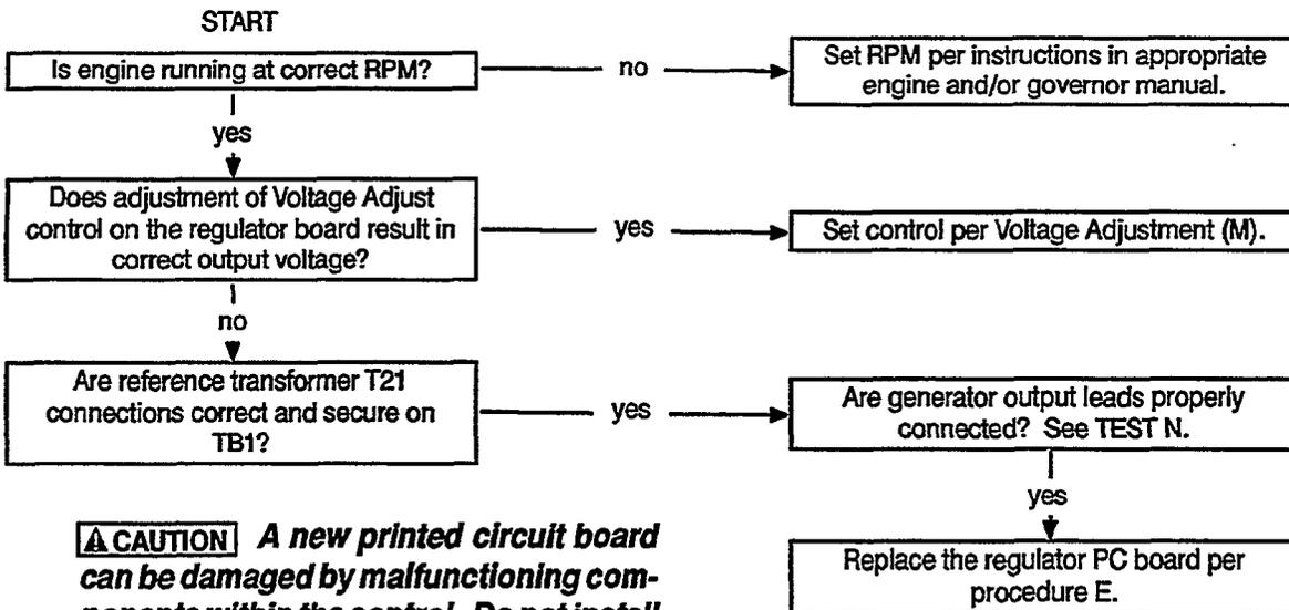
**CAUTION** A new printed circuit board can be damaged by malfunctioning components within the control. Do not install the new PC board until all other problems have been located and corrected.
