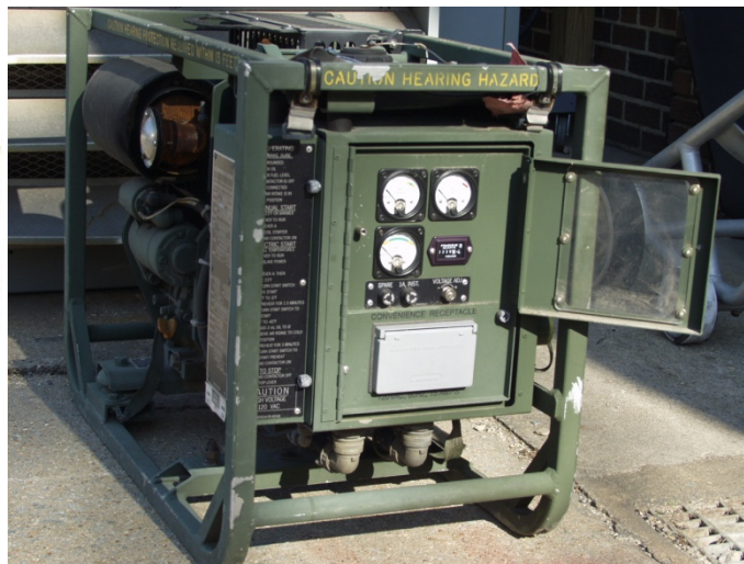
MEP-531A, 120 V, 60 Hz has an additional meter (frequency) and a convenience receptacle
