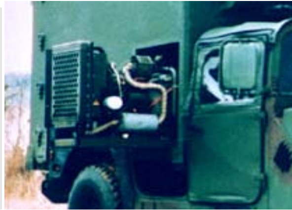
10 kW APU ready to slide into shelter. - front view -
