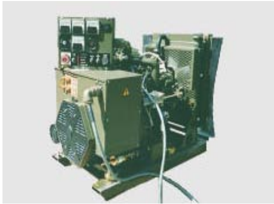
10 kW APU and control panel removed from shelter. – rear view --
