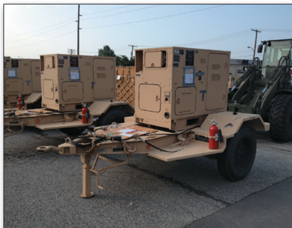
Photo credit: U.S. Army. AMMPS units being readied for fielding to Afghanistan.
