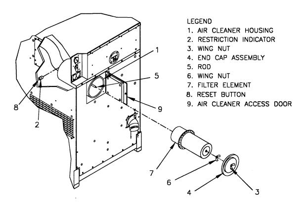
FIGURE 3-1. AIR CLEANER ELEMENT REPLACEMENT
