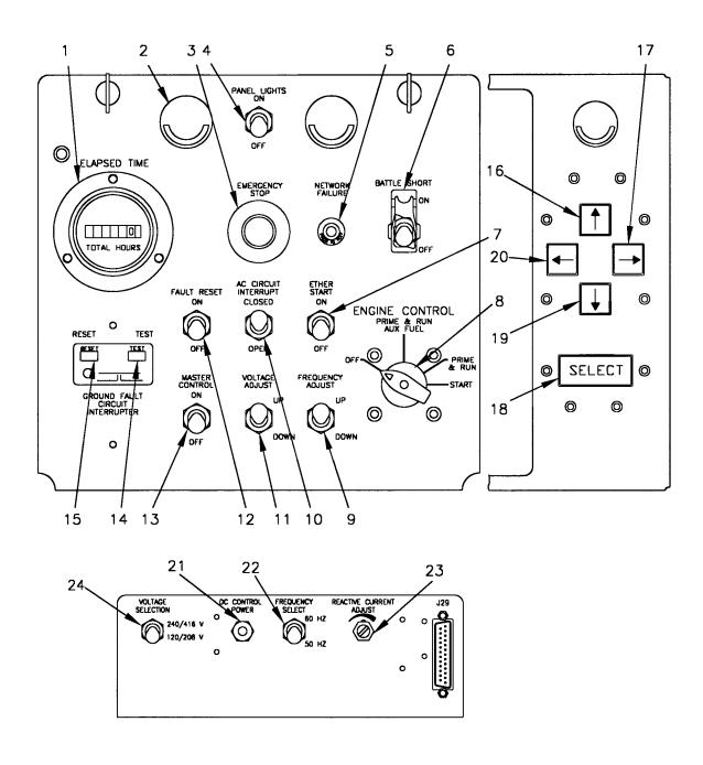
FIGURE 2-1. DCS CONTROLS AND INDICATORS
