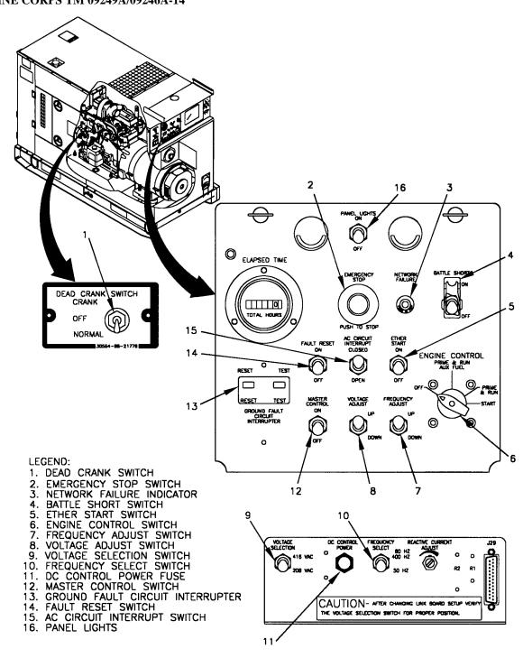
FIGURE 2-8. GENERATOR SET CONTROLS
