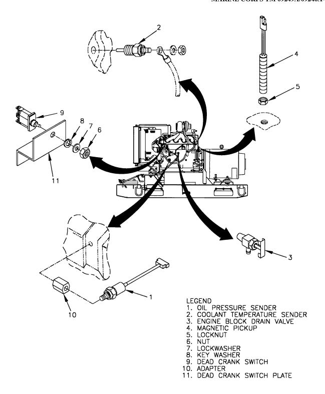
FIGURE 4-30. ENGINE SWITCHES AND SENDERS
