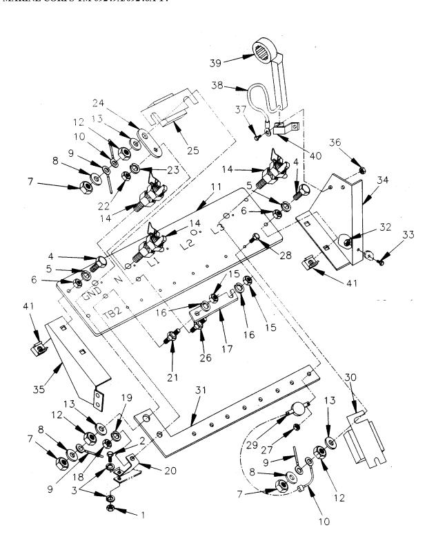
FIGURE 4-29. LOAD OUTPUT TERMINAL BOARD ASSEMBLY (SHEET 1 OF 2)
