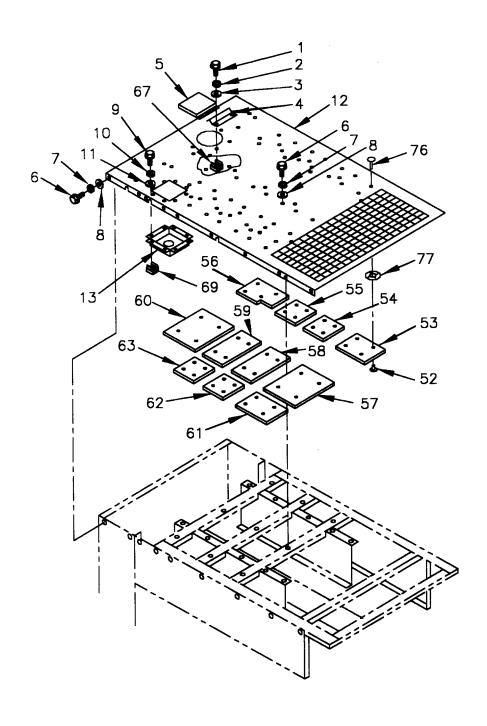
FIGURE 4-7. TOP HOUSING SECTION (SHEET 1 OF 3)
