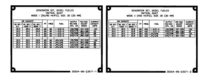
FIGURE 1-7. SET RATING IDENTIFICATION PLATE, MEP-805B AND MEP-815B
