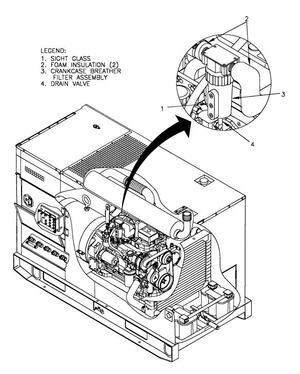
FIGURE 3-2 CRANKCASE BREATHER FILTER ASSEMBLY
