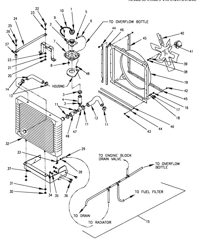
FIGURE 4-22. COOLING SYSTEM (SHEET 1 OF 2)
