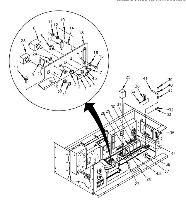
FIGURE 4-16. DCS CONTROL BOX FLOOR COMPONENTS (SHEET 1 OF 2)
