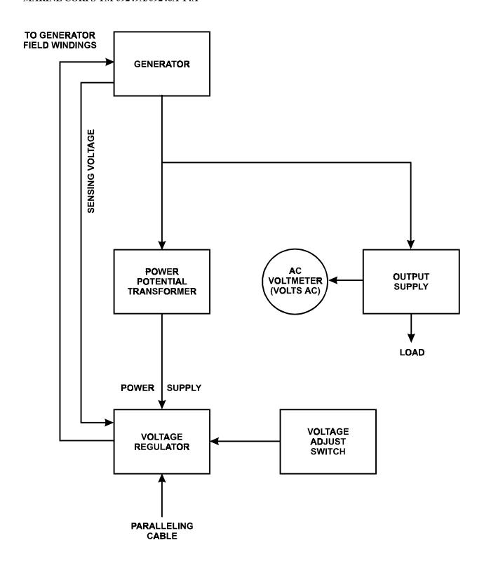
FIGURE 1-21. VOLTAGE REGULATION SYSTEM FLOW DIAGRAM
