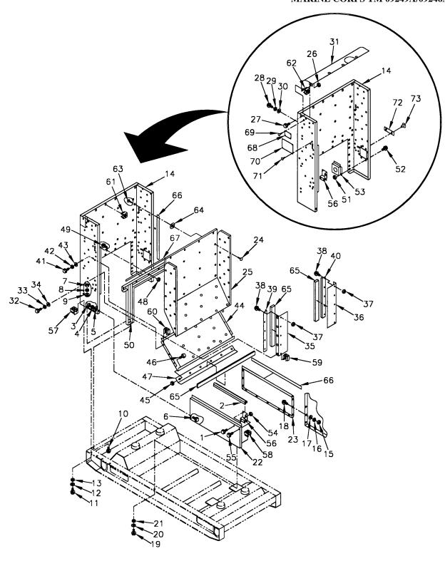
FIGURE 4-8. FRONT HOUSING SECTION (SHEET 1 OF 2)
