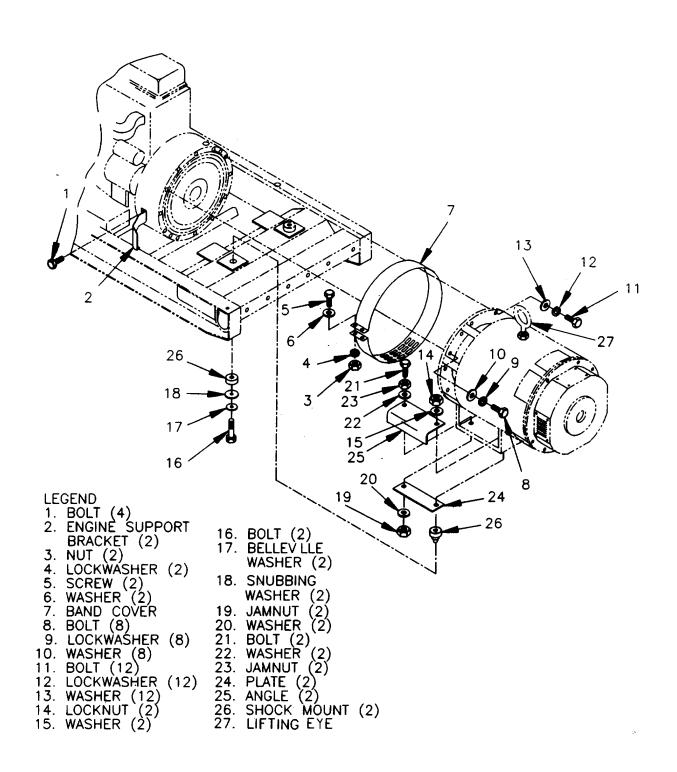
FIGURE 5-8. GENERATOR ASSEMBLY REMOVAL
