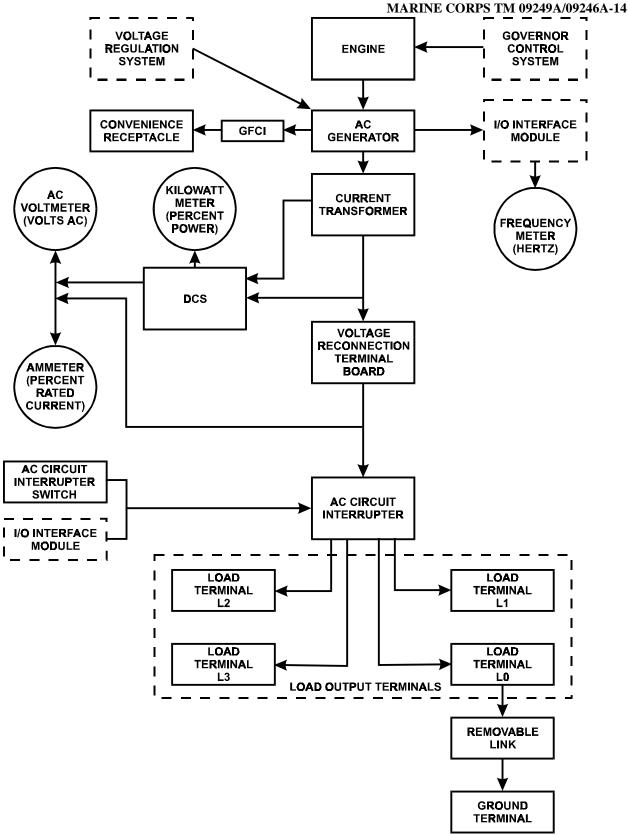
FIGURE 1-27. OUTPUT SUPPLY SYSTEM FLOW DIAGRAM
