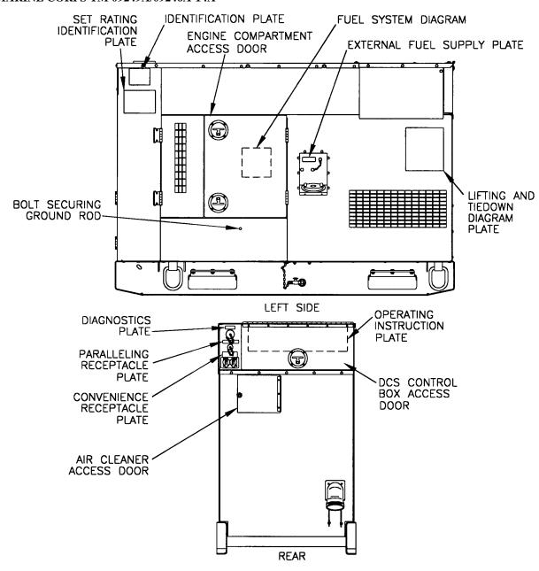
FIGURE 1-3. LOCATIONS OF DATA PLATES AND ACCESS DOORS (REAR AND LEFT SIDE)
