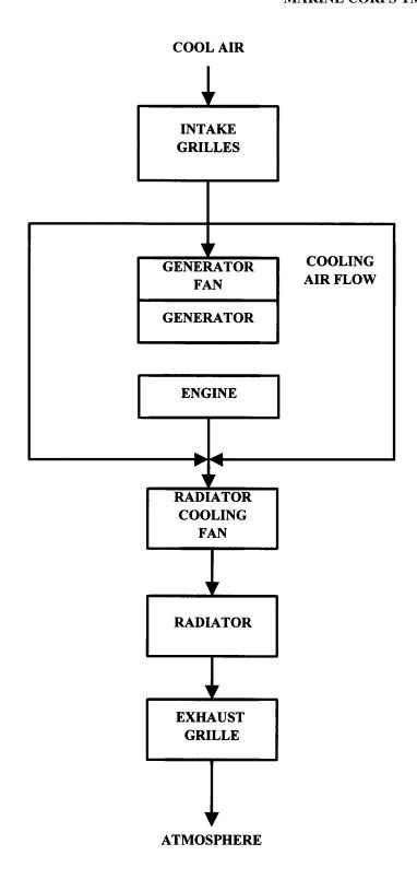
FIGURE 1-23. GENERATOR SET COOLING SYSTEM FLOW DIAGRAM
