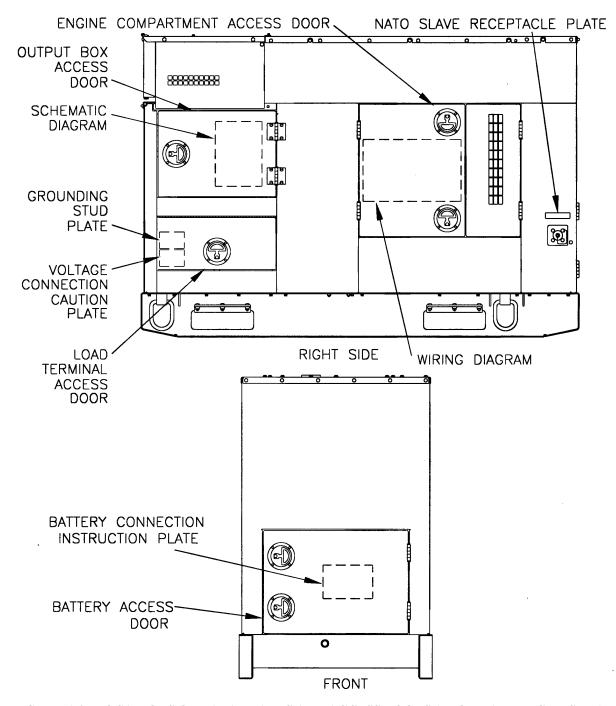
FIGURE 1-2. LOCATIONS OF DATA PLATES AND ACCESS DOORS (FRONT AND RIGHT SIDE)
