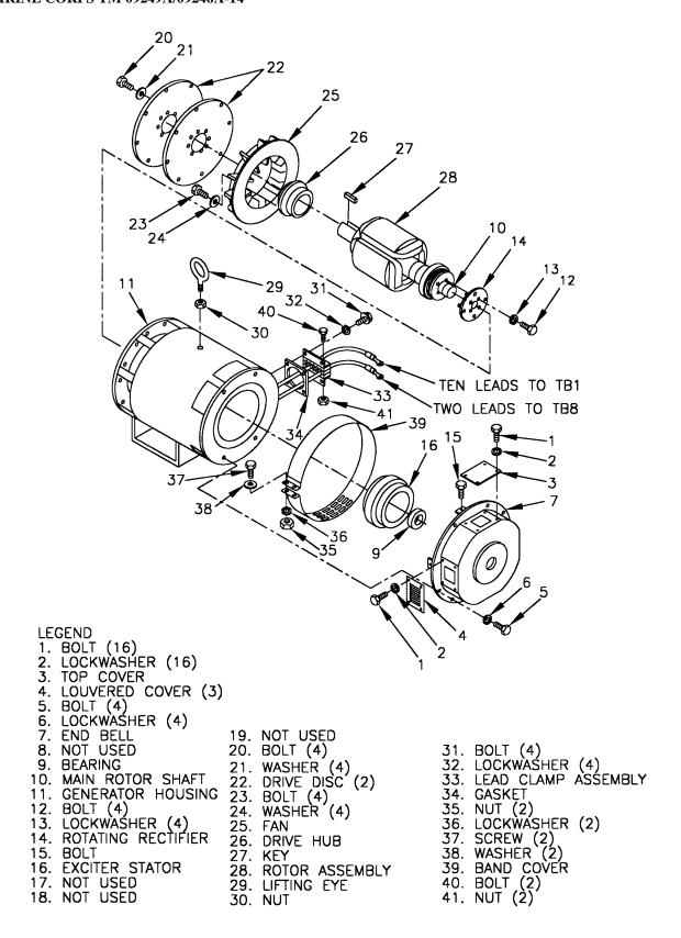
FIGURE 5-9. GENERATOR ASSEMBLY
