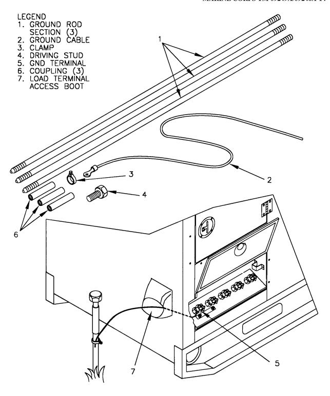
FIGURE 2-6. GROUNDING CONNECTIONS
