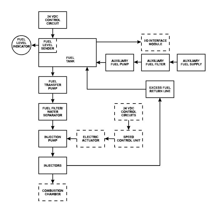
FIGURE 1-22. FUEL SYSTEM FLOW DIAGRAM
