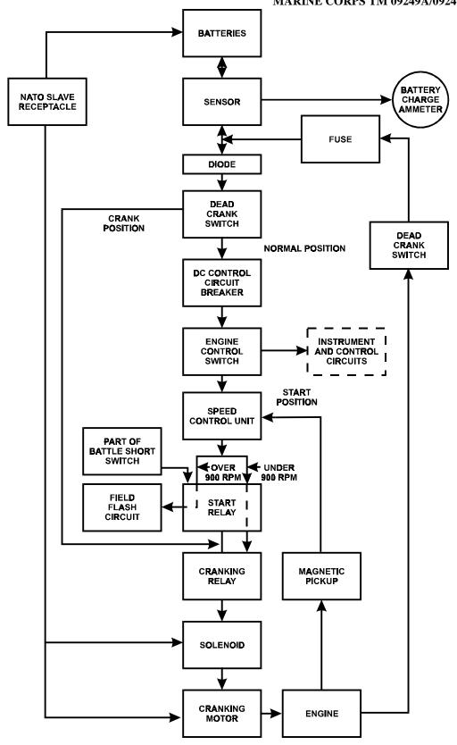
FIGURE 1-29. ENGINE STARTING SYSTEM FLOW DIAGRAM
