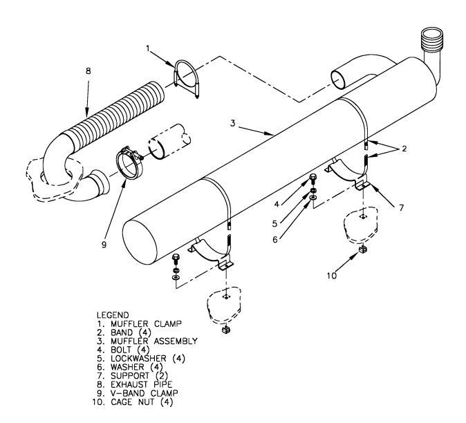
FIGURE 4-19. MUFFLER AND EXHAUST PIPE
