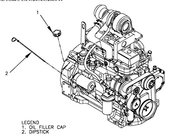
FIGURE 4-2. DIPSTICK AND OIL FILL CAP
