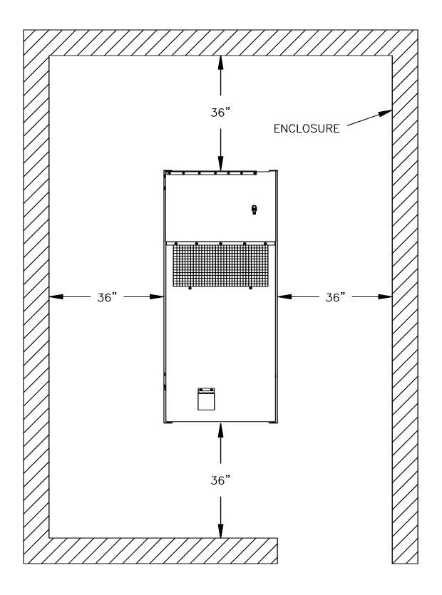
FIGURE 2-5. MINIMUM ENCLOSURE CLEARANCE MEASUREMENTS
