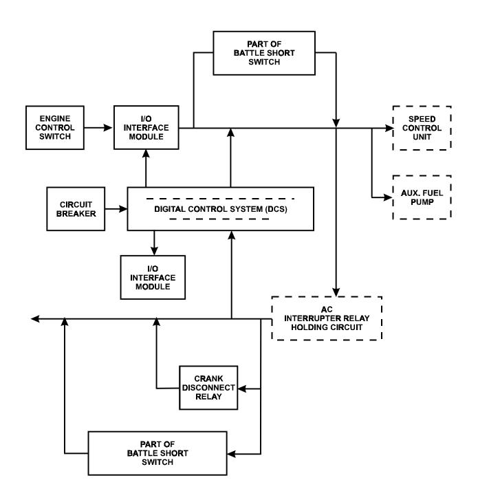
FIGURE 1-19. FAULT SYSTEM FLOW DIAGRAM
