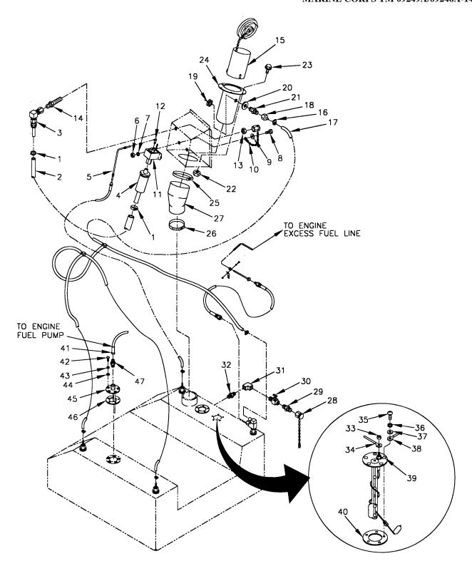
FIGURE 4-26. FUEL TANK FILLER NECK AND LOW PRESSURE FUEL SYSTEM (SHEET 1 OF 2)
