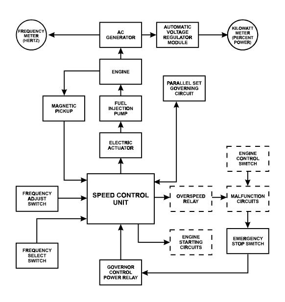
FIGURE 1-20. GOVERNOR CONTROL SYSTEM FLOW DIAGRAM
