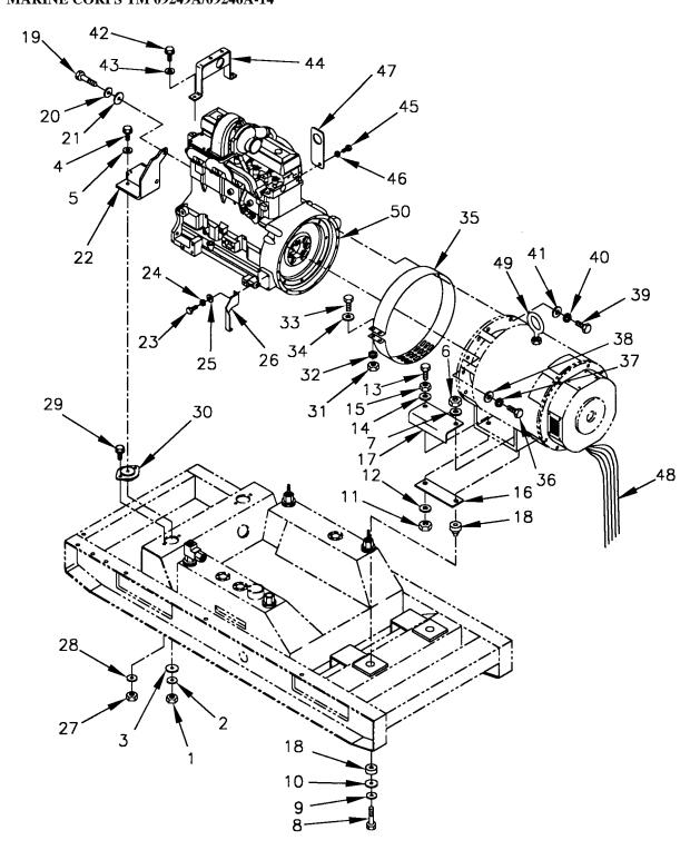
FIGURE 5-1. ENGINE AND GENERATOR ASSEMBLY (SHEET 1 OF 2)
