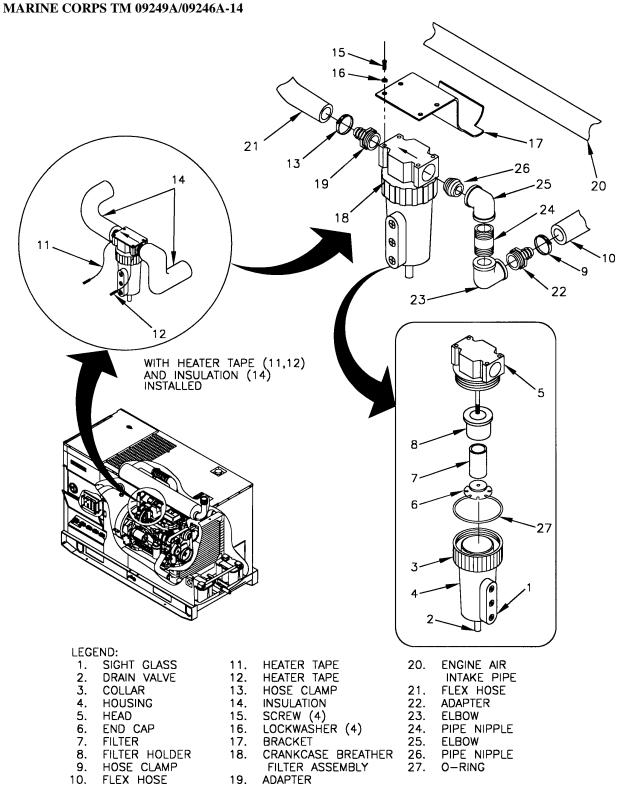
FIGURE 4-21. CRANKCASE BREATHER FILTER ASSEMBLY
