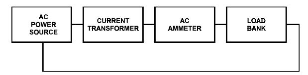
FIGURE 5-5. TESTING CURRENT TRANSFORMER
