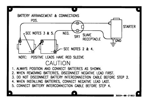
FIGURE 1-14. BATTERY CONNECTION INSTRUCTION PLATE
