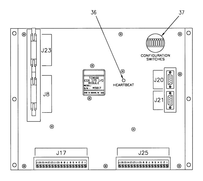
FIGURE 2-3. DIAGNOSTIC CONTROLS AND INDICATORS (SHEET 2 OF 2)
