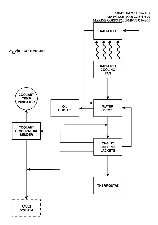
FIGURE 1-24. ENGINE COOLING SYSTEM FLOW DIAGRAM
