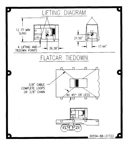
FIGURE 1-15. LIFTING AND TIEDOWN DIAGRAM PLATE
