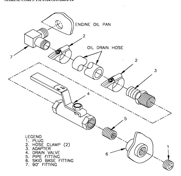
FIGURE 4-32. OIL DRAIN VALVE
