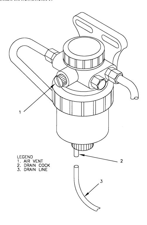
FIGURE 3-5. FUEL FILTER/WATER SEPARATOR
