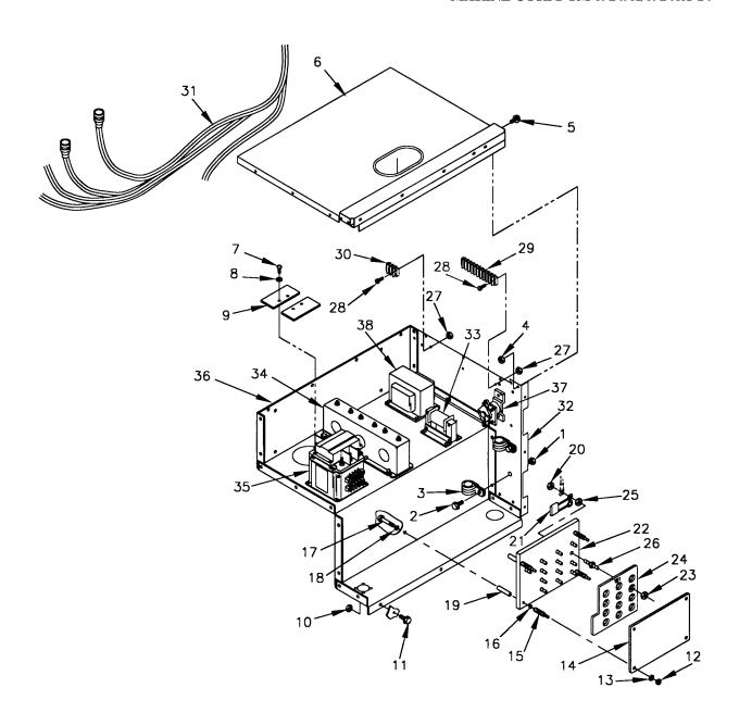
FIGURE 5-3. OUTPUT BOX ASSEMBLY (SHEET 1 OF 2)
